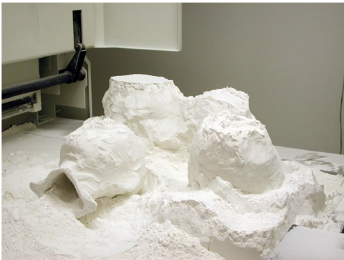
Photograph of the mummy models being removed from the Z-Corp machine. The plaster powder surrounding the models is recycled into the machine for the next print.
