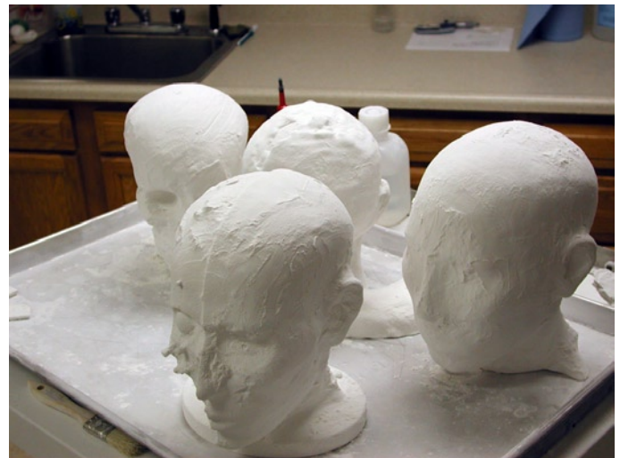
Photograph of the mummy models immediately after removal from the machine. Note the loose plaster powder on the surface; this will be removed with forced air during the finishing process.
