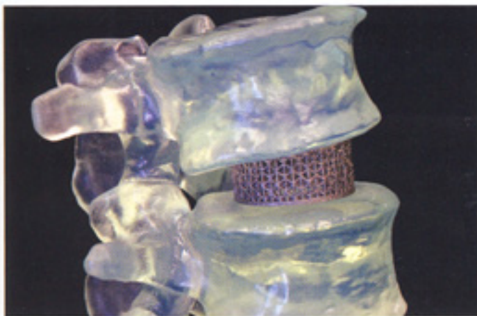
Figure 4: Model of the spine showing a lattice cage implant produced using the EBM manufacturing technique. (Courtesy Medical Modeling LLC)
