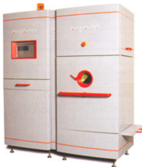
Figure 1: The Electron Beam Melting manufacturing method is carried out using a high power electron beam and a strong vacuum, ensuring fast throughput and reliable chemical specifications for Ti6Al4V-ELI parts. (Courtesy Arcam AB)
